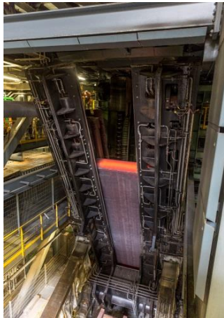
Picture 3: The continuous caster CC 6 already today underlines Dillinger's leading role in the production of high-quality continuous cast slabs.
