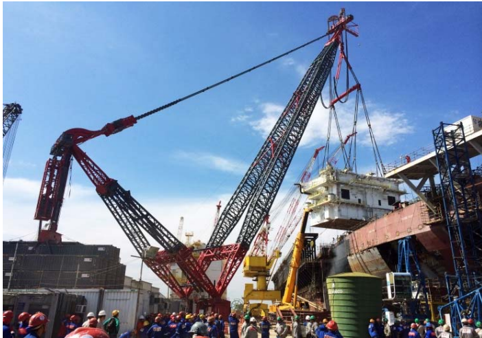
Figure 5: With a maximum boom height of almost 200 metres, load of 4,300 tonnes and a load moment of 196.000 tonne-metres, ALE's AL.SK190 became the world's largest capacity land-based crane.
