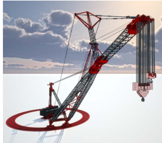
Figure 6: The fixed jib consisting of ultra-high-strength DILLIMAX steel serves as an extension of the boom and can, with its length of up to 100 metres, lift a maximum of 3,400 tonnes.
