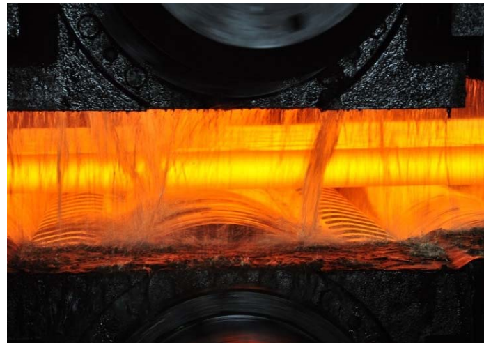
Figure 8: The application of rolling forces of 11,000 tonnes during rolling homogenises DILLIMAX plates down to their centre.
