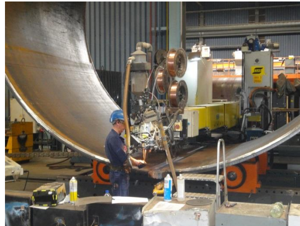
Picture 4: The formed plates are welded together internally and externally by a longitudinal weld.
