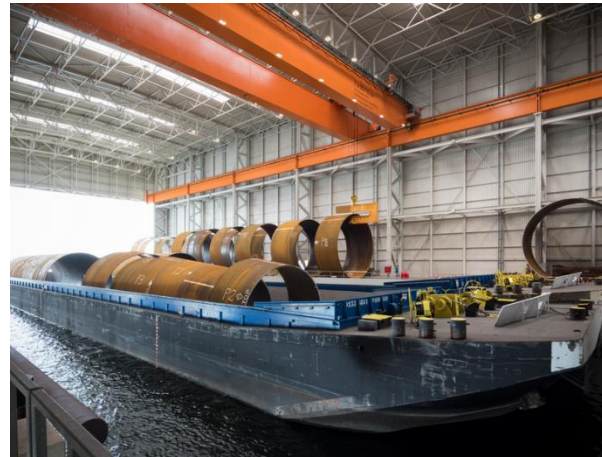
Picture 13-14: The monopiles or shell sections made of Dillinger steel are transported by ship from Roermond to shipyards or to the Rotterdam factory.
