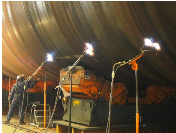
Picture 8: Up to four circumferential welds are made simultaneously by four welding heads, which are controlled by a single system operator.
