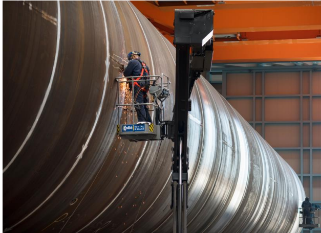
Picture 9-10: At the Roermond site, the large shell sections are assembled into XL monopiles.
