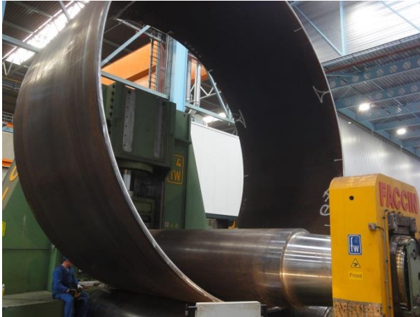
Picture 5: After each welding process, the shell sections, which are up to 11 meters in diameter, are calibrated in a ring roller.
