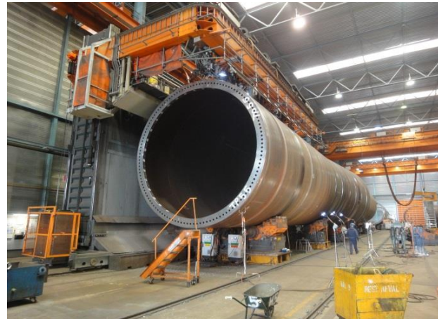
Picture 11-12: Sif manufactures XL monopiles from thermomechanically rolled steels from Dillinger in thicknesses of up to 140 millimeters.
