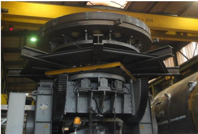
Image 11: Monobloc housing: for the largest and, at up to a maximum of 25 tonnes, heaviest unit in the TBM, Dillinger supplies heavy plates of up to 240 millimetres in thickness.
