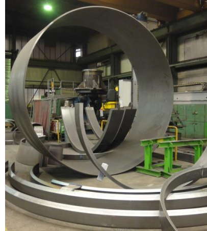
Images 9-10: For each drive system, Herrenknecht installs up to ten spacer, support and adapter rings with diameters of three to eight metres and an item weight of 15 tonnes, each fabricated from Dillinger heavy plates.
