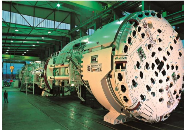
Image 4: 450 metres long, 3,000 tonnes in weight, 9.43 metres cutting diameter: Sissi, the longest Herrenknecht TBM yet, headed the Gotthard Base Tunnel using heavy plates from Dillinger.
