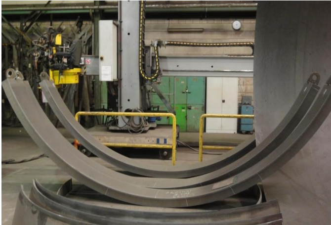
Images 9-10: For each drive system, Herrenknecht installs up to ten spacer, support and adapter rings with diameters of three to eight metres and an item weight of 15 tonnes, each fabricated from Dillinger heavy plates.
