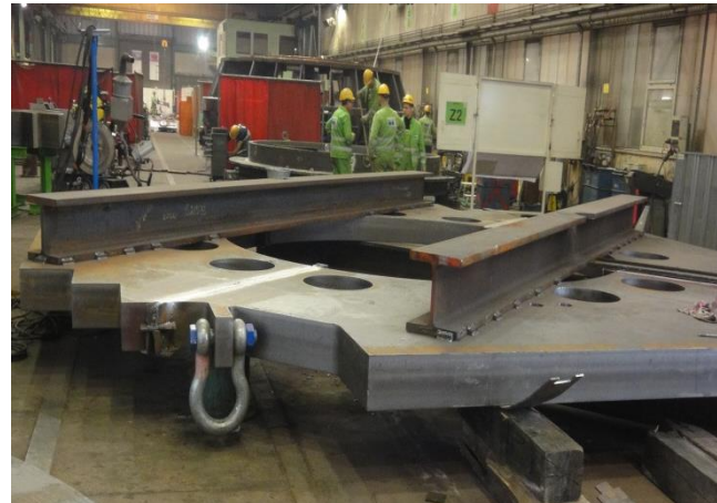
Image 8: : To assure stabilisation, Herrenknecht fits I-beams to the back plate of the gearbox housing, which consists of four segments of Dillinger steel.
