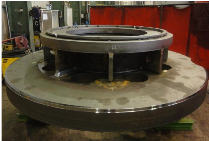
Image 7: 100 percent Dillinger steel: extremely thick plates from Dillinger are indispensable for the gearbox housing, the dimensions of which are a function of torque and thrust.
