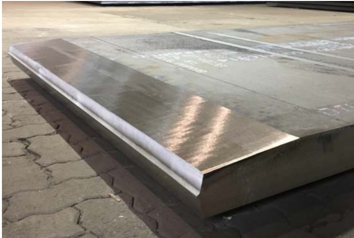
Picture 1: The innovative weld-edge preparation of Dillinger's Heavy Fabrication Division combines a very flat tapering and a tulip-shaped edge for very thick and long plates.
