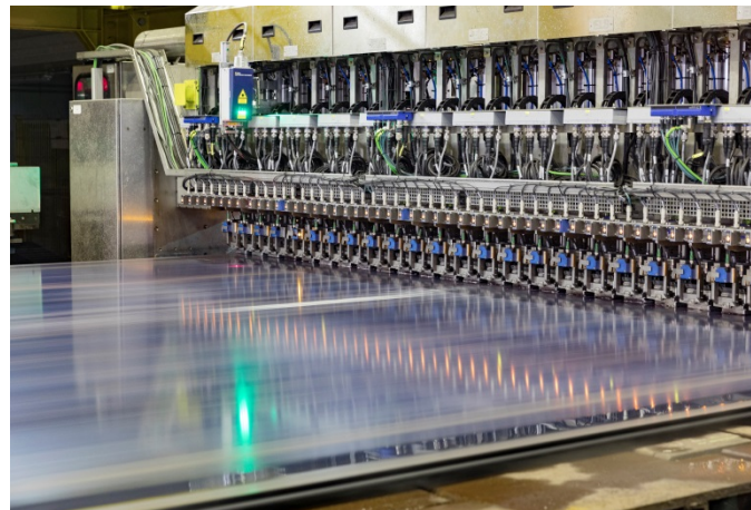
Picture 4: Dillinger's D-TECT technology inspects plates in order to ensure that hard spots are one hundred percent non-existent.
