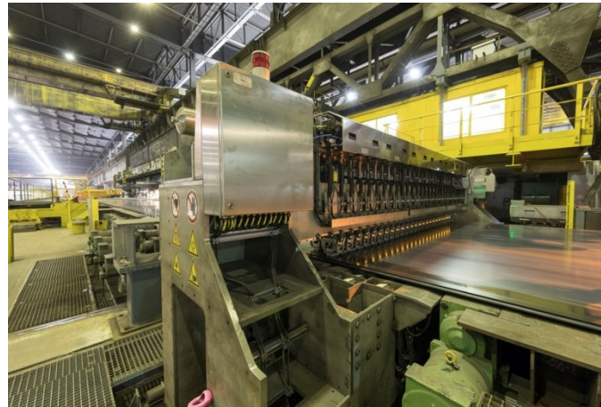
Picture 2: The newly developed D-Tect inspection technology from Dillinger makes it possible – even during the production process – to detect hard spots on plates.
