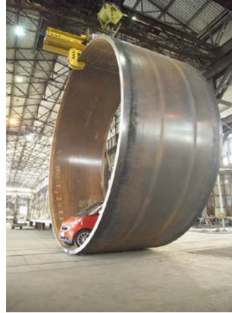
Picture 10: Shell section with a diameter of 7,500 mm
