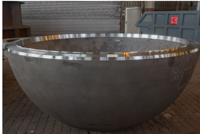
Picture 16: Hemispherical one-piece vessel head with turned edge
