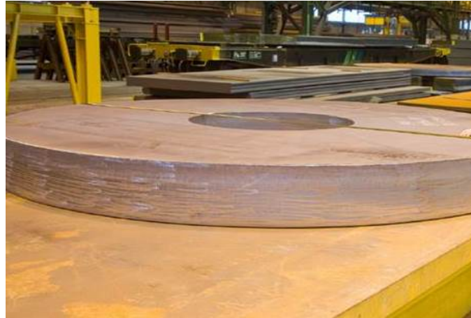
Picture 2: Large, heavy ring segment with a thickness of 305 mm for a hydropower station
