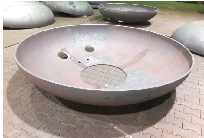
Picture 24: Customised package delivery: here, a one-piece head with holes for connection components
