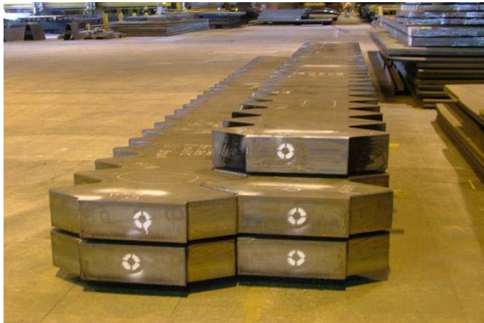
Picture 3: Racks up to 250 mm thick for a jack-up rig
