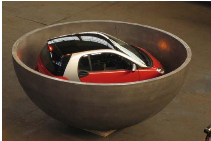
Picture 15: Hemispherical one-piece vessel head with a diameter of 3,450 mm
