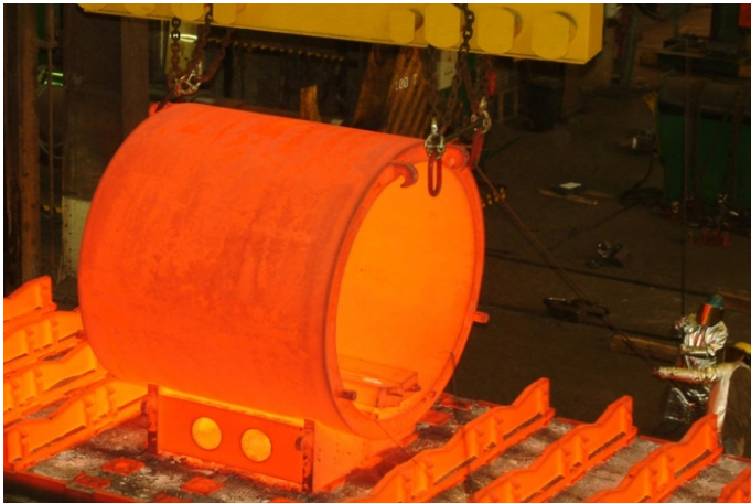
Picture 11: Thermal treatment of a shell section with wall thickness of 240 mm
