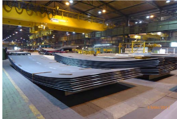
Picture 6: Ready-to-install, tailor-made components – edge-prepared and roll-bent for tank container construction
