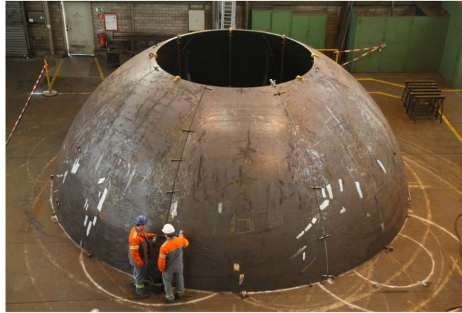
Picture 18: Trial fit-up of a hemispherical multi-segment vessel head with a diameter of 10,000 mm and a wall thickness of 25 mm
