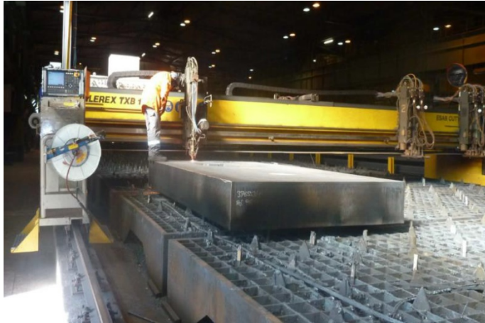
Picture 1: Thermal cutting of heavy plate in thicknesses up to 430 mm and item weights up to 45 t
