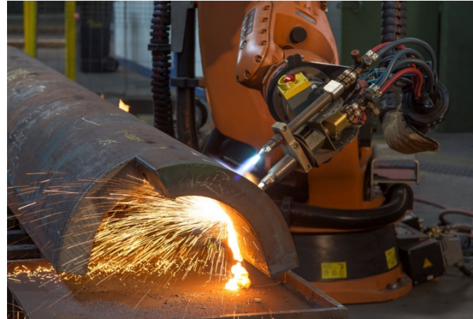
Picture 22: Robot-supported edge preparation on a chord with a wall thickness of 120 mm made of steel grade S690Q mod.
