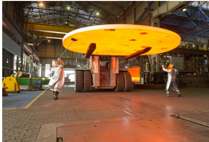
Picture 12: Pre-heated, round blank before forming into a thick-walled hemispherical one-piece vessel head with a diameter of 3,600 mm
