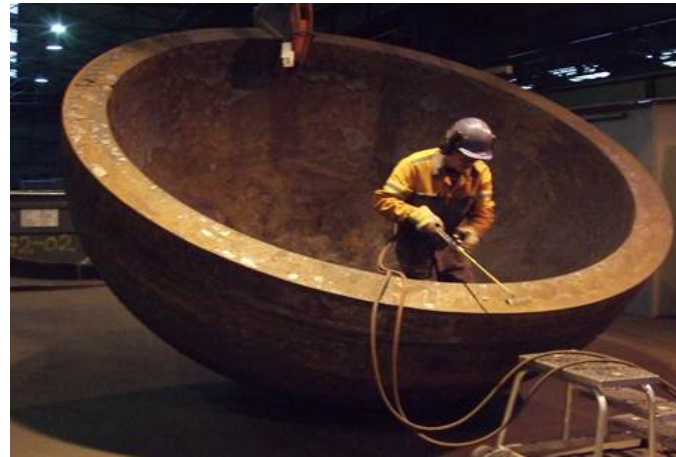
Picture 14: Hemispherical one-piece vessel head with a wall thickness of 200 mm
