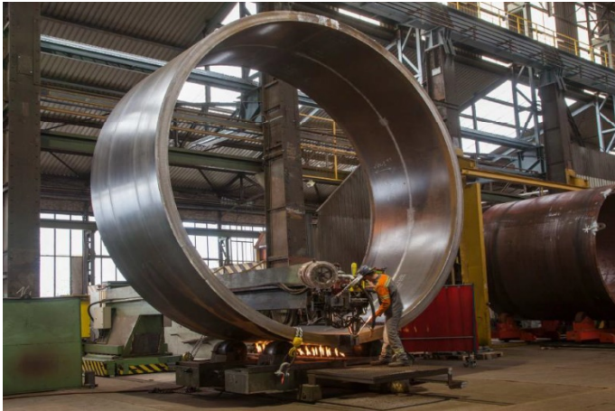
Picture 9: Welding a cold-formed shell section with two longitudinal welds; wall thickness 180 mm
