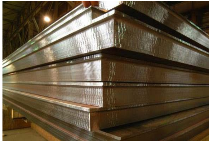
Picture 4: Heavy plates with customised preparation of machined welding seams
