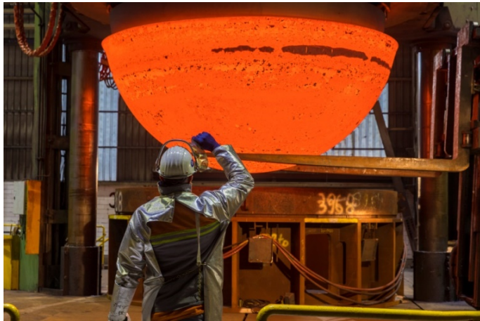
Picture 13: Forming a hemispherical one-piece vessel head with a diameter of 3,800 mm
