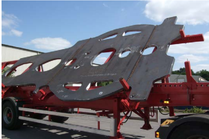
Picture 5: Precision flame-cutting parts delivered "just-in-time" for construction machinery and mechanical engineering
