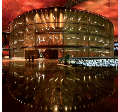
Picture 9: The facade of the Beijing Opera House is clad in Xinghai, a special blended mesh with aluminium weft and stainless steel warp anodised in two gold tones.
