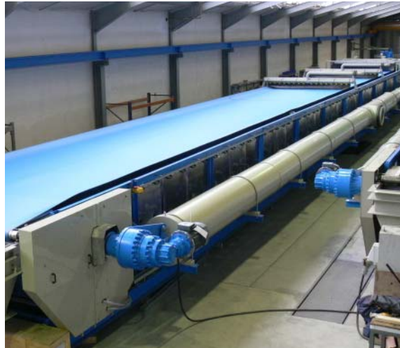
Picture 2: The VACUBELT® filter belt 2015 from GKD has already proven its worth in the field of FGDP gypsum dewatering over many years.
