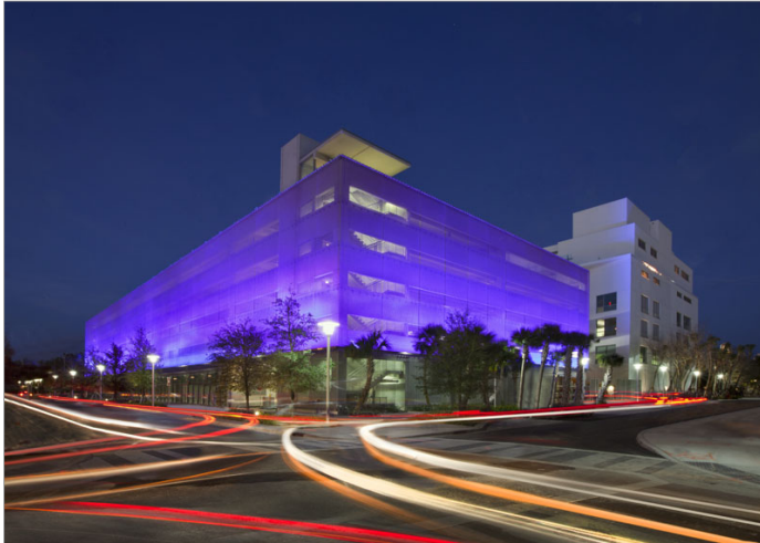
Picture 5: At night, the 3-D effect on the stainless steel mesh is accentuated by LED illumination.
