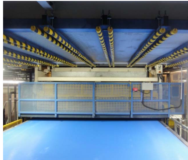
Picture 2: The CONDUCTIVE® 7690 forming belt by GKD, was at the heart of the mesh and fabric specialist's trade fair appearance.
