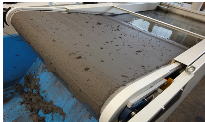
Picture 4: MAXFLOW Belt Filter with self-cleaning endless stainless steel mesh belt by GKD.
