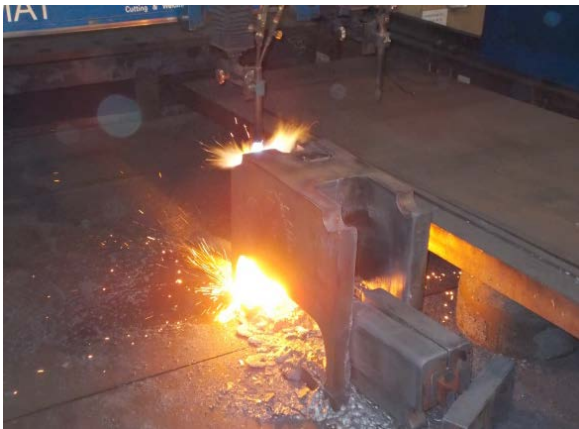
Picture 3: Without resorting to milling, the thermal cutting specialists produced the complex geometries exactly to the customer's specifications.
