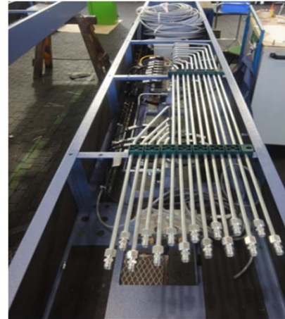
Image 11: The supply lines for hydraulics, pneumatics and lubrication are accommodated in the installation profiles.
