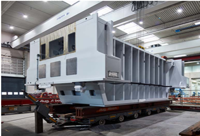
Images 1 - 2: 3,620 mm high, 4,950 mm long and 7,950 mm wide: ANDRITZ Kaiser commissioned Jebens, as the leading specialist in large, heavy flame-cut parts and blanks and complex welded constructions, with the production of the press table.
