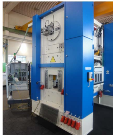
Images 9 - 10: The compact design of the servo presses is thanks to the integration of oil tank and hydraulic units in the machines.
