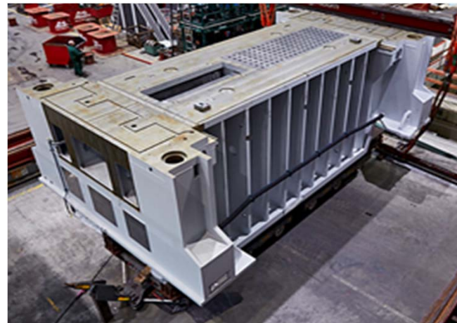
Images 1 - 2: 3,620 mm high, 4,950 mm long and 7,950 mm wide: ANDRITZ Kaiser commissioned Jebens, as the leading specialist in large, heavy flame-cut parts and blanks and complex welded constructions, with the production of the press table.
