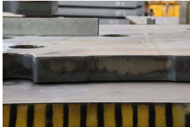
Picture 13+14: For the straightening of the 120-millimetre-thick sheets of the high-strength steel with the flame, the proven expertise of the master aligner at Jebens was needed.
