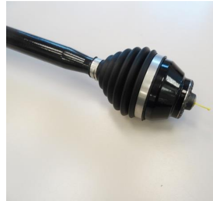
Pictures 8-10: Neapco relies on the in-depth material and process know-how of Pallas GmbH & Co. KG to coat the outer joints and their spur gearing.
