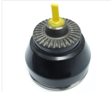
Pictures 8-10: Neapco relies on the in-depth material and process know-how of Pallas GmbH & Co. KG to coat the outer joints and their spur gearing.
