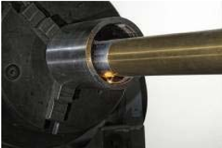
Picture 3: iClad® achieves high-quality coatings even when things get tight (diameters down to 30 mm).
