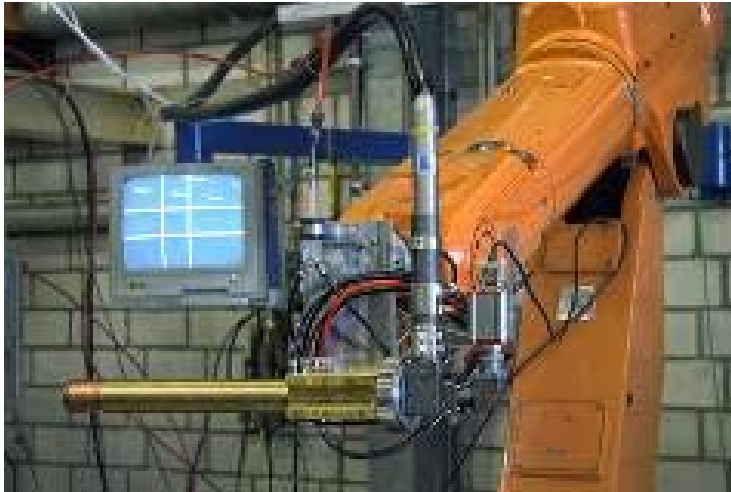
Picture 1: The modular structure of iClad® allows different heads to be attached for different coating challenges.
