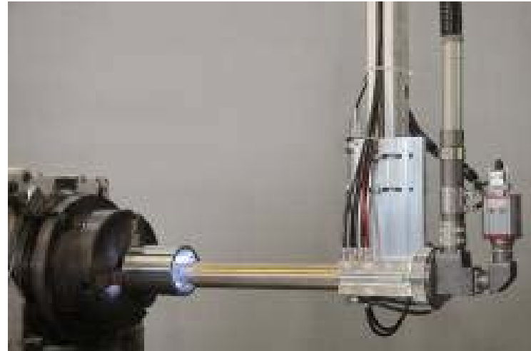
Picture 2: For many inaccessible parts that are subject to wear, iClad® covers the complete range of internal surface treatment needs.
