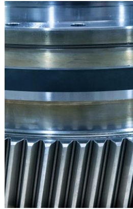
Picture 10: The coating of the large 700 kilogram components must be absolutely pore-free, have a surface roughness of R_a 0.4 \mu\text{m} and, after finishing, be ground perfectly smooth.
