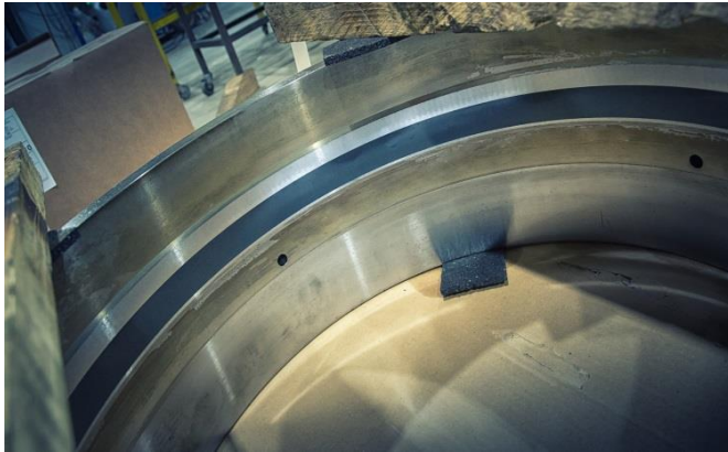
Picture 9: Pallas coats both the external and internal seats of the gears in one clamping.
