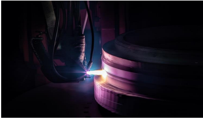
Picture 5-6: A refractory ceramic compound in powder form is injected into a plasma flame burning at a temperature of 18,000°C, where this feedstock melts in microseconds and is propelled by the kinetic energy against the surface of the workpiece.
