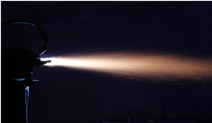
Picture 7-8: Particles of a refractory ceramic coating – with high dimensional precision and reliable reproducibility – form a dense, highly adhesive layer on the substrate to be coated.
