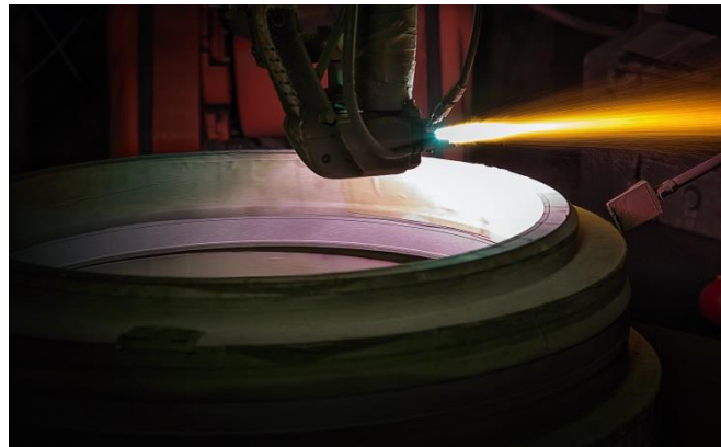
Picture 7-8: Particles of a refractory ceramic coating – with high dimensional precision and reliable reproducibility – form a dense, highly adhesive layer on the substrate to be coated.
