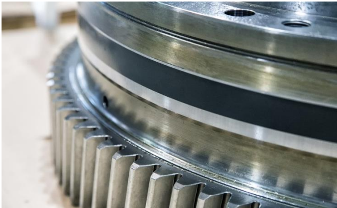
Picture 11-12: That's why the sealing seats are internally and externally machined and polished to their final dimensions in the last stage of processing, so that the complete system has the required tightness.
