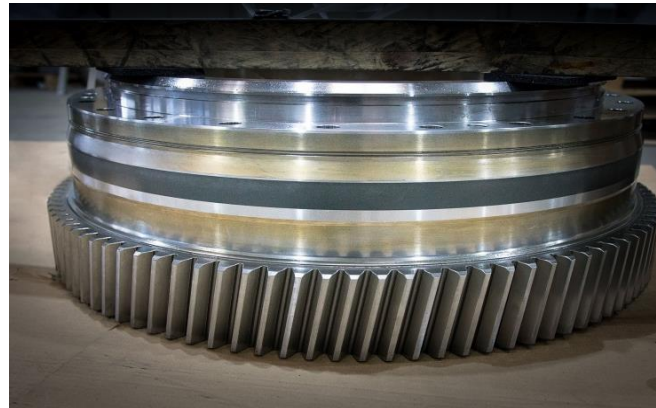
Picture 11-12: That's why the sealing seats are internally and externally machined and polished to their final dimensions in the last stage of processing, so that the complete system has the required tightness.
