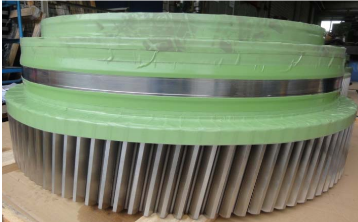
Picture 10: The uncovered spots inside and outside of this pinion gear drive will be thermal coated, sanded and burnished.
