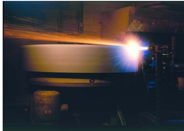
Picture 3-4: In wire flame spraying practically any coating material that is available in wire form can be deposited, while electric arc spraying is a cost-effective way of using electrical energy to create firmly bonded, wear-proof surfaces that are resistant to high temperatures and oxidation.
