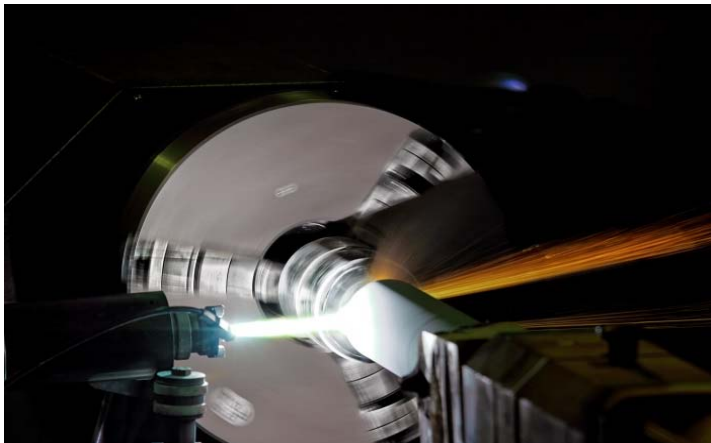
Picture 7: The combination of such a high level of kinetic energy with a relatively low level of thermal energy is optimal for creating very firmly bonded, homogeneous and dense hard metal coatings.
