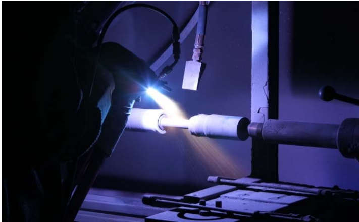
Picture 5: In the up to 20,000 °C-hot plasma flame, atmospheric plasma spraying even processes refractory ceramics and their compounds into extremely hard, wear resistant coatings.
