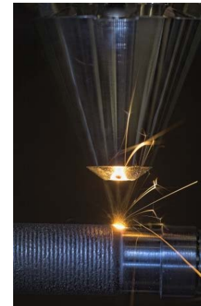
Picture 8-9: Laser processes are appropriate for improving the surface properties of expensive, highly stressed components.
