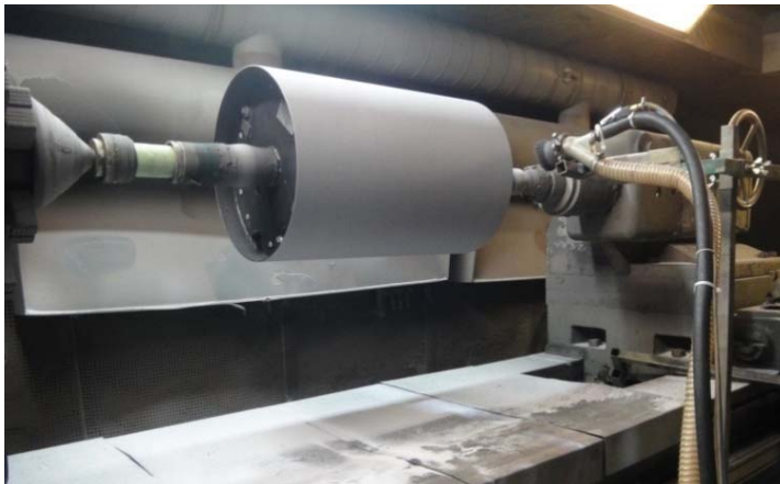
Picture 12: The castors are processed with a mobile sandblast device.
