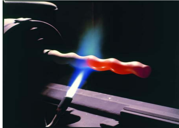
Picture 2: Powder flame spraying creates coatings with thicknesses up to several millimetres.
