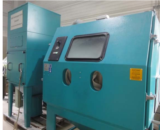
Picture 11: In its own sandblast cabin Pallas prepares castors for brake dynamometers for the coating process.
