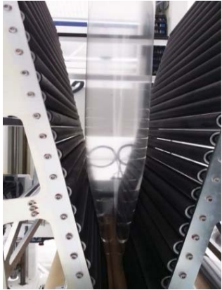
Pictures 7+8: Biaxially oriented multi-layer blown film in a single work process (Triple Bubble®)
