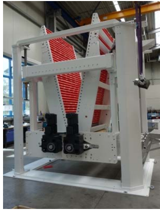
Picture 14: Roller board for flattening during the manufacturing process
