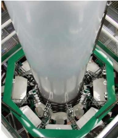
Picture 4: Air-cooled blown film ( Smart Bubble®) with calibration cage
