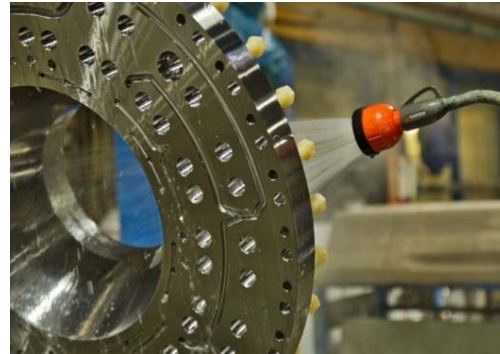
Picture 2: Multi-stage degreasing process after masking of threads
