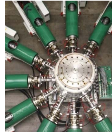
Picture 6: Smart Bubble® with 9-layer extruder
