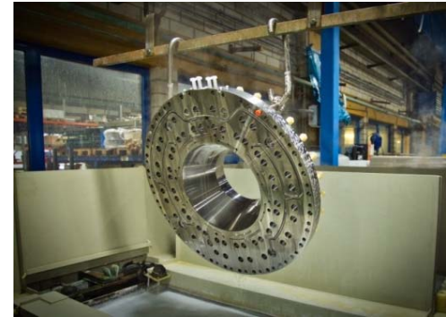
Picture 3: Coating thickness dependent on how long mandrel stays in bath
